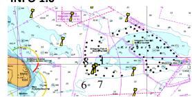
Within the windfarm a seaweed farm has been established. The site is marked by 4 yellow buoys. The lines and buoys are in the surface in the seaweed farm at Danish Kriegers Flak and navigation within the marked area should be avoided.
